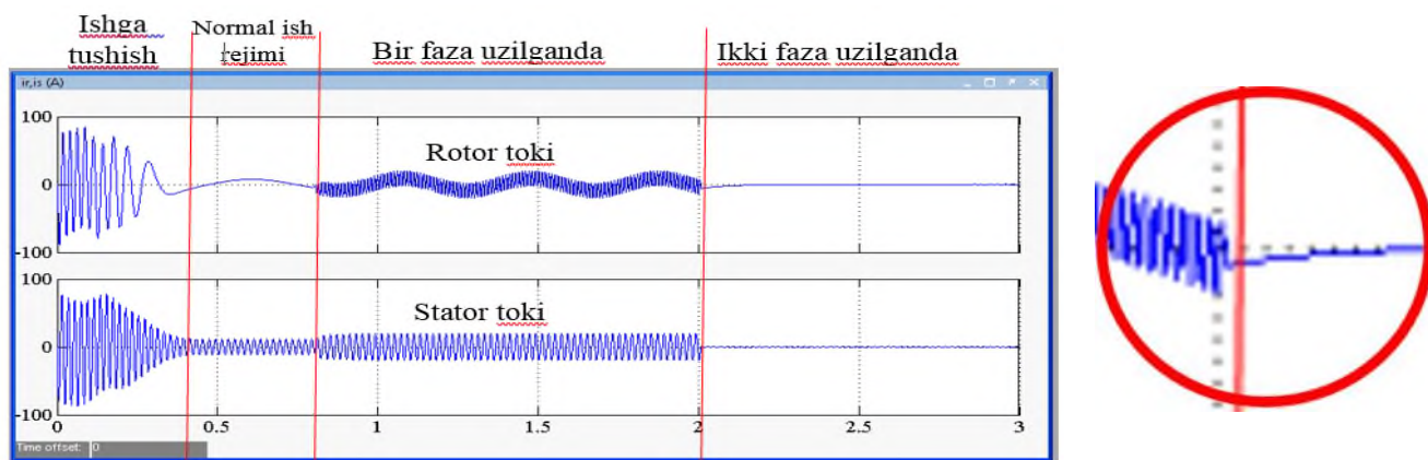
3-rasm. Matlab immitasion modelda olingan asinxron motorning stator va rotor toklari ossilogrammalari
