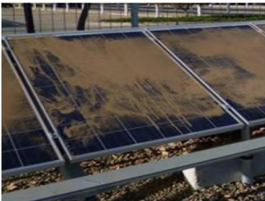
Figure 1. Solar panel state of pollution
