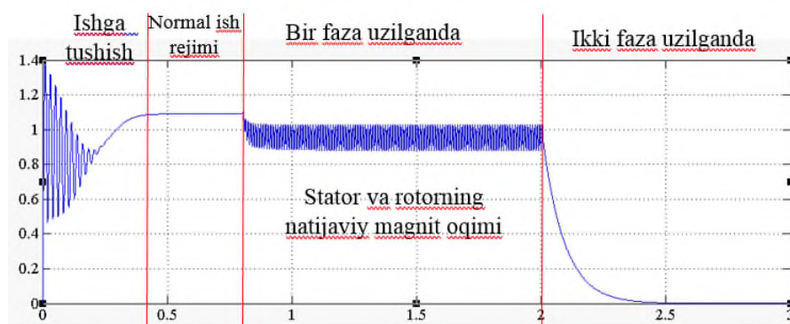
5-rasm. Matlab imitatsion modelda olingan asinxron motorning stator va rotor natijaviy magnit maydonining ossilogrammasi
