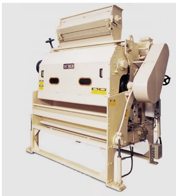
3-rasm. Turkiyaning Sumer 180 saw linter mashinasi
