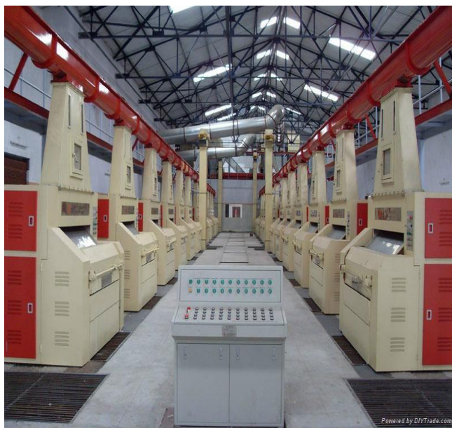
2-rasm. Xitoy paxta tozalash ko'xonasidagi MR 160-11C rusumli linter mashinalarining linterlash jarayoni
