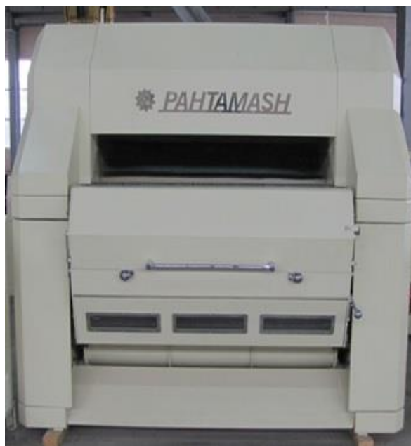
4-rasm. O'zbekistondagi 5-ЛПП rusumli linter mashinasi
