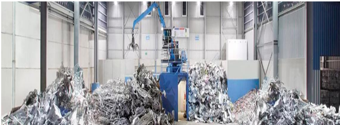
2-rasm. Ikkilamchi alyuminiy chiqindilarini saralash
