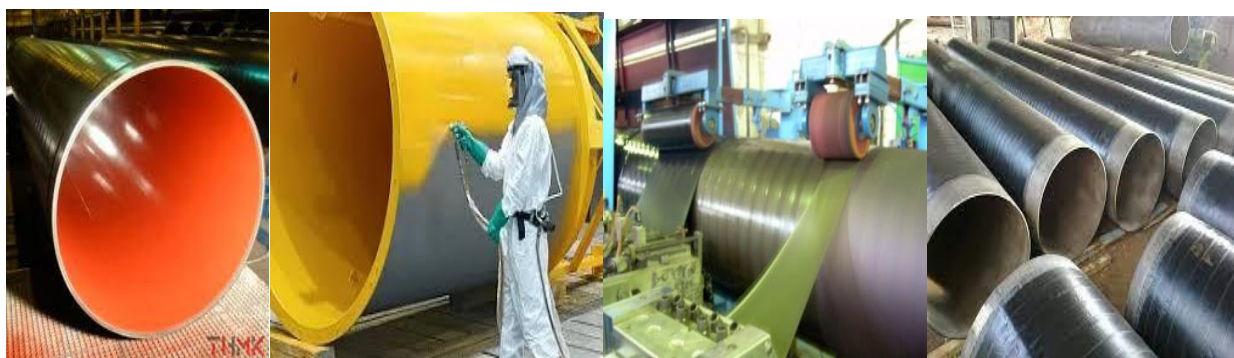
Figure 1. Types of anti-corrosion coatings for main pipes
