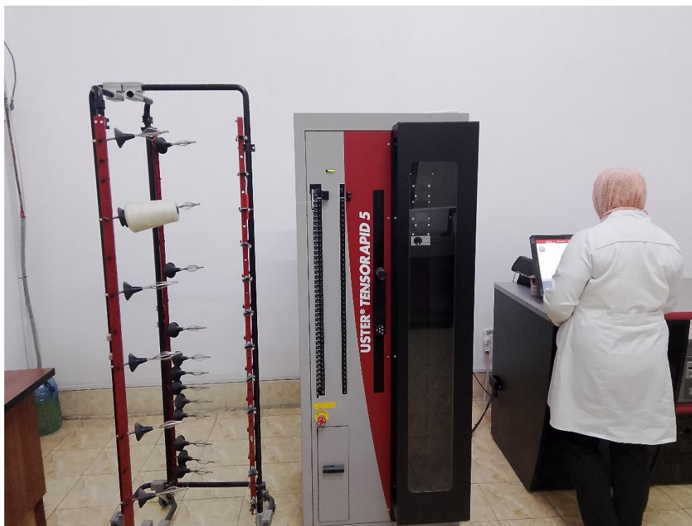
4- rasm. USTER-TESTER asbobida jun va akril tolalaridan yigirilgan iplarning test tahlillari
