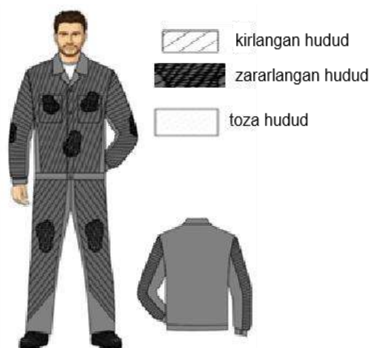
1-rasm. Payvandchi maxsus kiyimining shlak va uchqunlardan zararlanish topografiyasi
